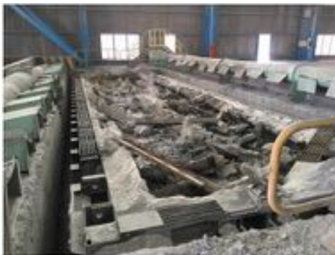
Figure 5: Starting the demolishing of the lining material in the de-lining shop
