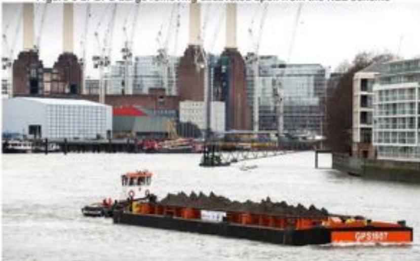
Figure 3-2: GPS barge removing excavated spoil from the NLE scheme
